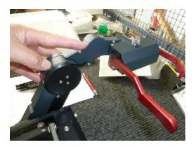
6. Lift Cover vertically to remove from chassis.
