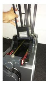
3. Remove both hotel locking bars from Chassis (two screws each side)
