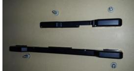
4. Remove the six cover retaining screws.( three each side)
