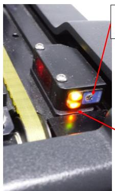
Sensor sensitivity, can be controlled by adjusting the sensitivity screw located on the front of Sensor
