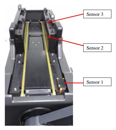
To Access The two plate sensors located at the hotel positions it will be necessary to remove the outer cover ( see cover removal procedure) and also to remove the sensor cover plate.
